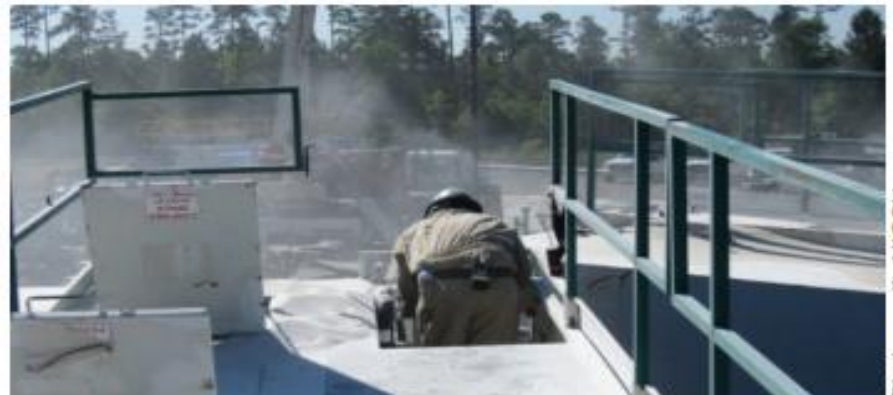
Silica dust cloud by worker delivering sand from sand mover to transfer belt.
