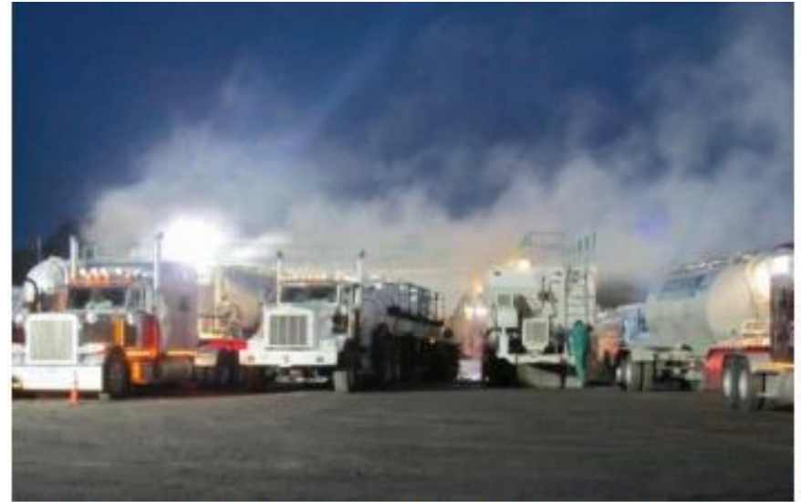
Silica dust clouds from delivery trucks loading into sand movers.
