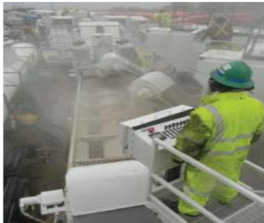
Silica dust by worker conducting sand transfer operations. Photo shows sand mover and transfer system.
