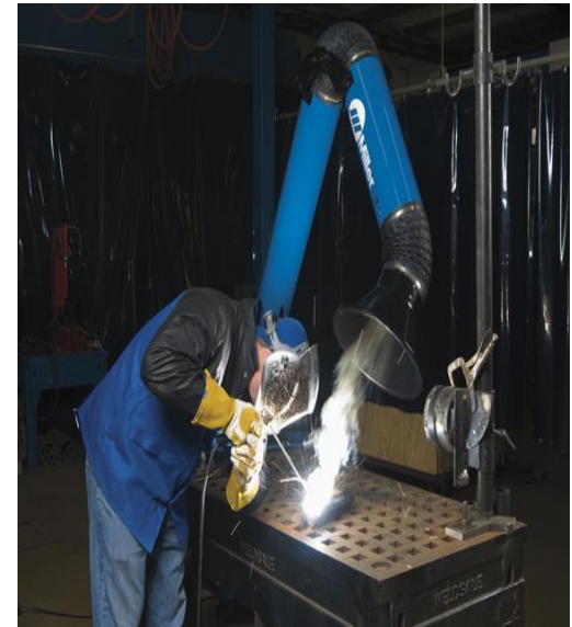
Trunk hose draws the fume away from a welder's breathing zone
