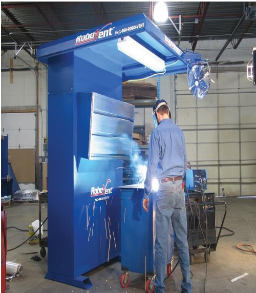
Backdraft welding bench is good for welding small parts
